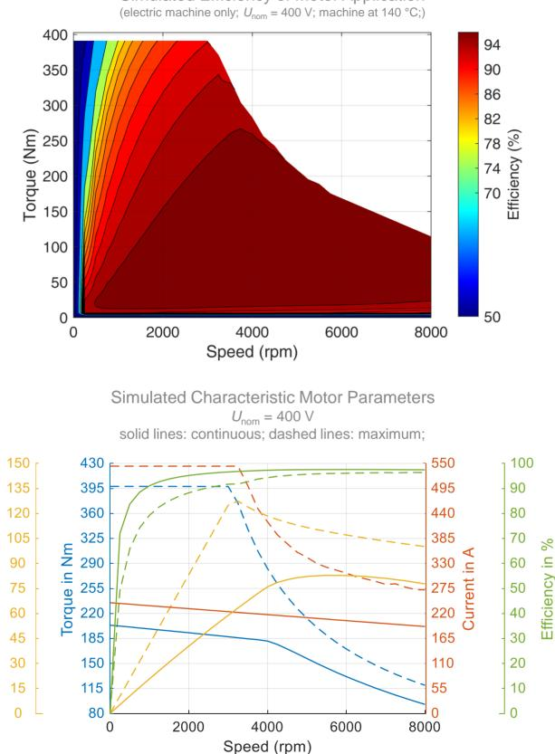
Simulated Efficiency of Motor Application (electric machine only;  $U_{nom} = 400 \text{ V}$ ; machine at 140 °C;)
