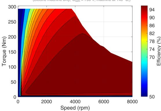
Simulated Characteristic Motor Parameters  $U_{\text{nom}} = 700 \text{ V}$  solid lines: continuous; dashed lines: maximum;
