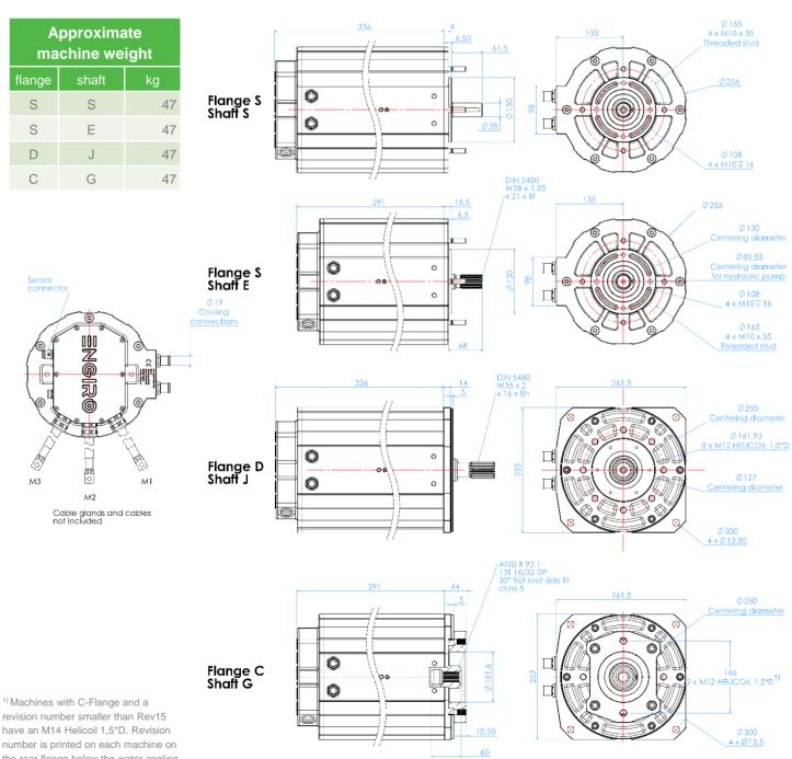
have an M14 Helicoil 1,5\*D. Revision number is printed on each machine on the rear flange below the water-cooling
