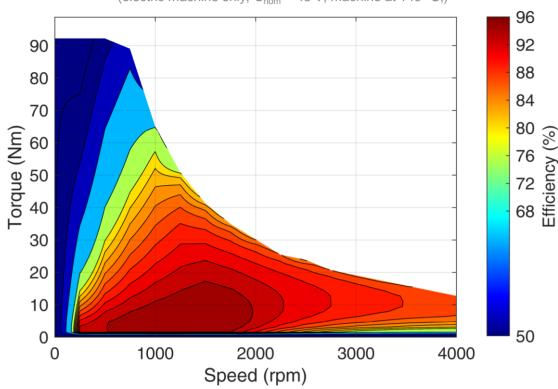
Simulated Characteristic Motor Parameters  $U_{\text{nom}} = 48 \text{ V}$  solid lines: continuous; dashed lines: maximum;
